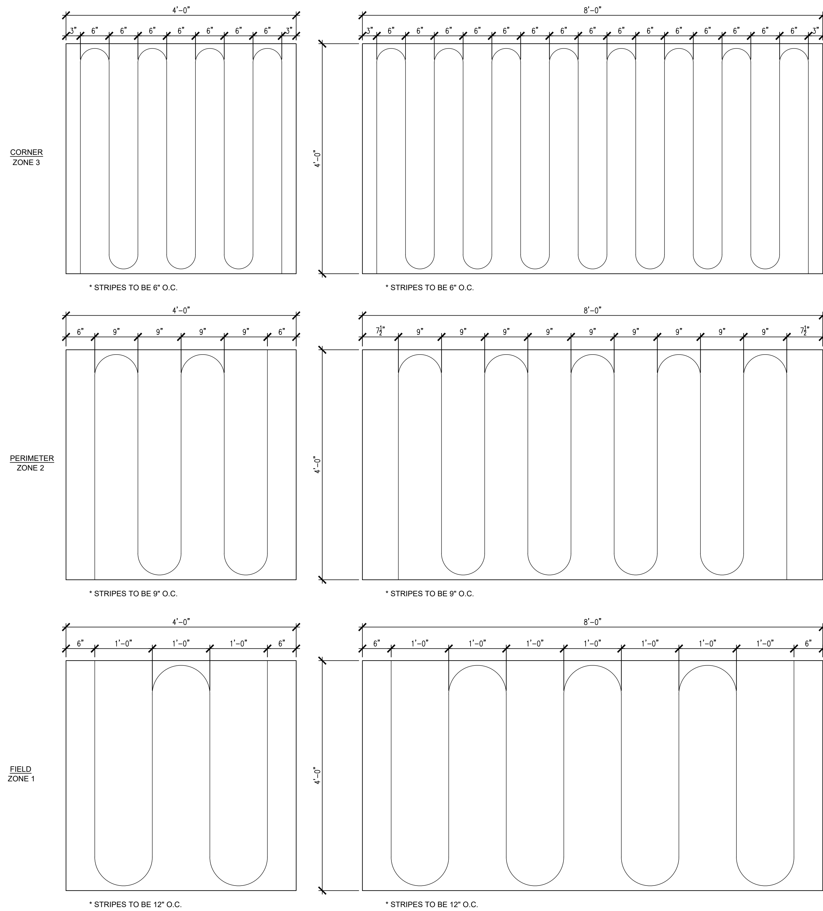
3 EXAMPLE ADHESIVE ATTACHMENT PATTERNS NOT TO SCALE
